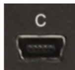
Figure 3.1. The W20B Mini-USB Local Console Port
