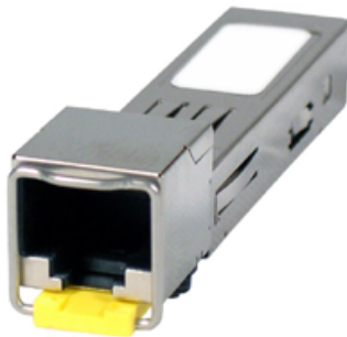
Figure 5.4. An Example of an SFP 1000 Base TX Module
