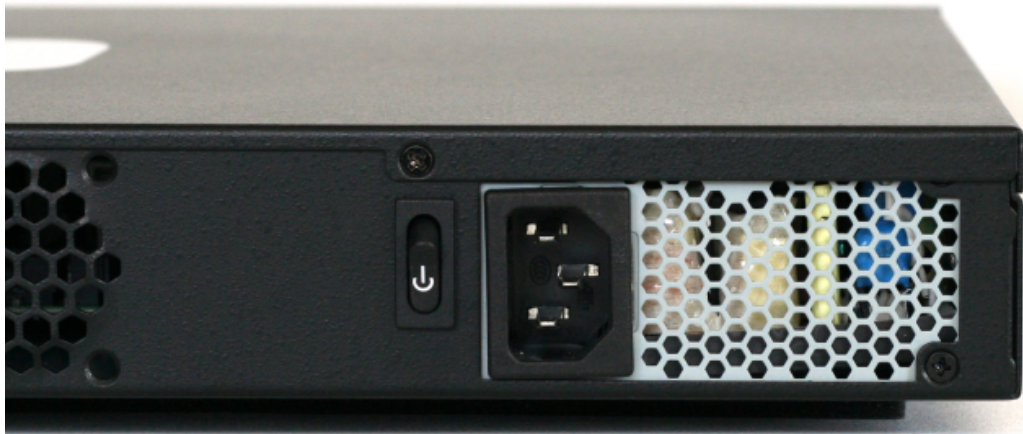
Figure 3.3. W30 Power Switch and Power Inlet Socket
