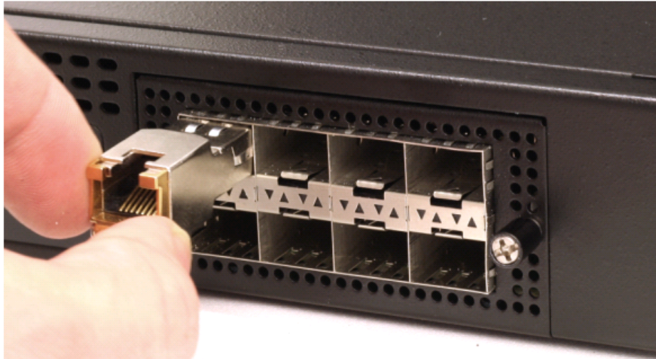
Figure 6.5. Insertion of a Gigabit SFP Module
